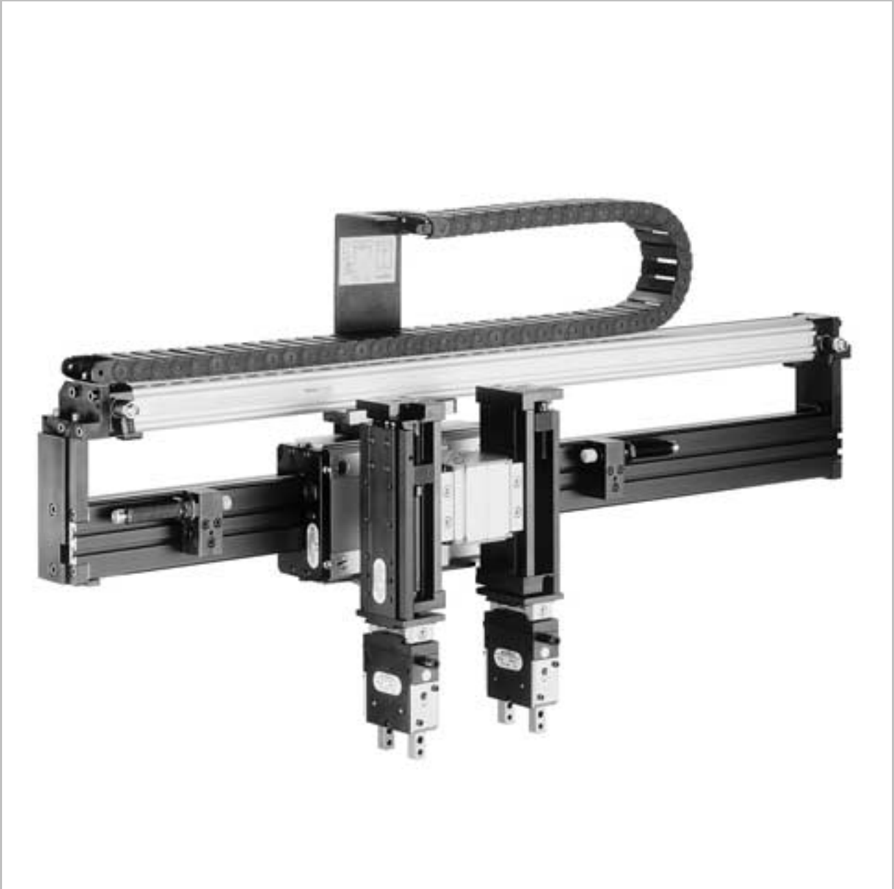
Transposition unit in portal design; two Compact Slides KSD, with Dual-Acting Parallel Grippers GPD, are built onto a Portal Slide PS with a TP-66-40 and an SLL-55-40.
